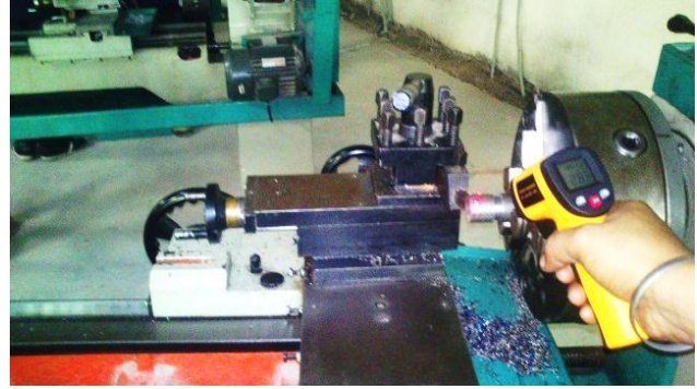
Fig 2: Measurement of temperature using infrared thermometer
