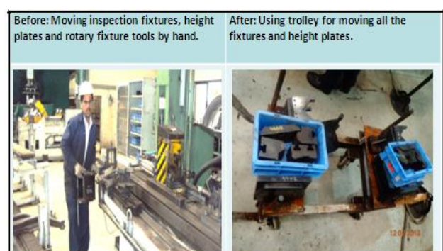
Figure 5 Use of trolley for moving Inspection fixtures & Rotary fixture
