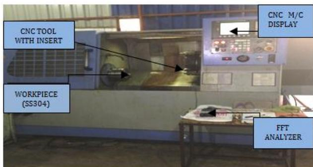
**Fig.1** Experimental setup of CNC Lathe Turning Operation
