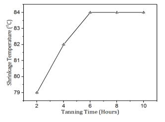
**Fig.3** Effect of time on the Ts of wet white leather (dose of SHMP = 12% of pelt weight, pH of the bath = 3)
