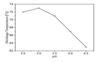
**Fig.1** Effect of pH on the Ts of wet white leather (Tanning time = 2 hour, dose of SHMP = 8% of pelt weight)
