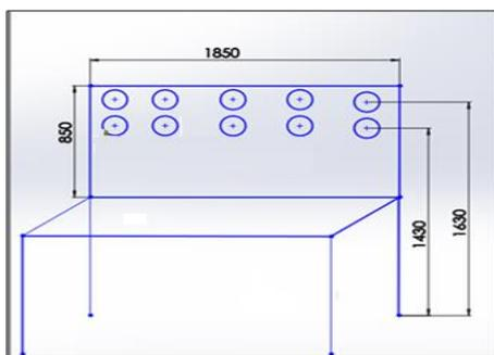
Figure 2 Layout of the holes for pressure gauges on Universal Test Bench
