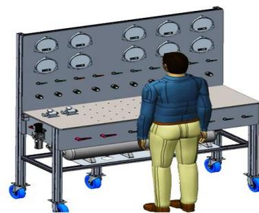
Figure 4 Universal Test Bench CAD Drawing
