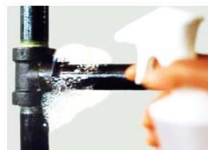
**Figure 10** Soap water test method
