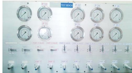
Figure 9 Notations of port on Universal Test Bench
