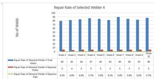
Fig. 5 Repair rate for Selected Welder 4
