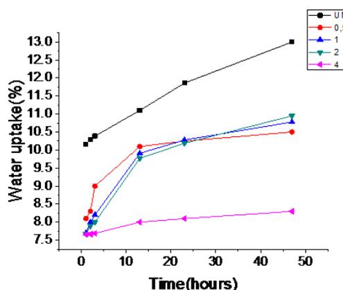
**Fig.8**Water uptake of treated and untreated samples verses time (CF<sub>6</sub>)
