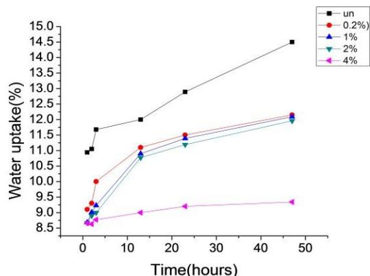
**Fig.9** Water uptake of treated and untreated samples verses time (CF<sub>4</sub>)
