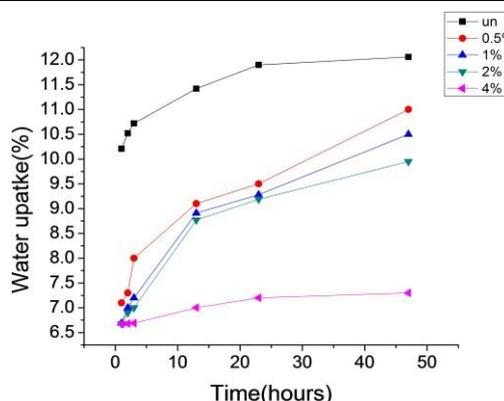
**Fig.7** Water uptake of treated and untreated samples verses time (CF<sub>8</sub>)
