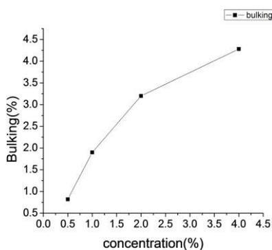
**Fig.6**Concentration of the solution verses bulking effect (CF<sub>4</sub>)
