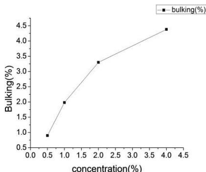
**Fig.6** Concentration of the solution verses bulking effect (CF<sub>6</sub>)
