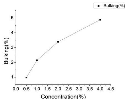
**Fig.5**Concentration of the solution verses bulking effect (CF<sub>8</sub>)
