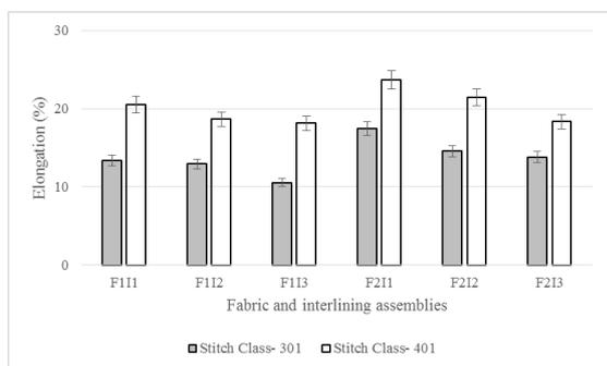
Figure 14: Elongation comparison of developed fabric and interlining assemblies' samples.
