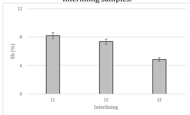
**Figure 9:** Eb% (elongation at break) variations of fabricated interlining samples.
