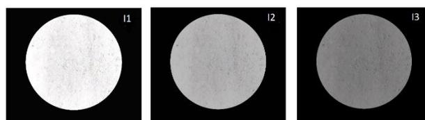
**Figure 4:** Image of fabricated interlining (I1) bleached 100% cotton waste material; (I2) 50% cotton/50% polyester mixed waste materials; (I3) 75% polyester/25% cotton mixed waste materials.
