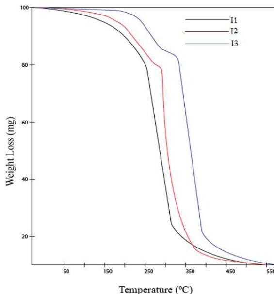
**Figure 11:** TGA of fabricated interlining samples.
