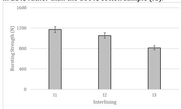
**Figure 10:** Bursting strength variations of fabricated interlining samples.
