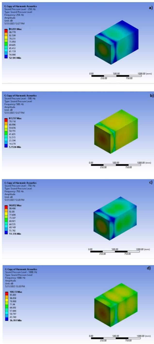
**Figure 8.** FFT Analysis on Ansys for Frequency [a] 250Hz, [b] 500Hz, [c] 750Hz, [d] 1000Hz at constant sound pressure source 100dB with composition 40% Coco Peat and 60% of Recycled Rubber
