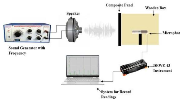
**Figure 4.** Schematic diagram of experimental setup of acoustic measurement
