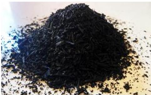
**Figure 2.** Secondary material recycled rubber.
